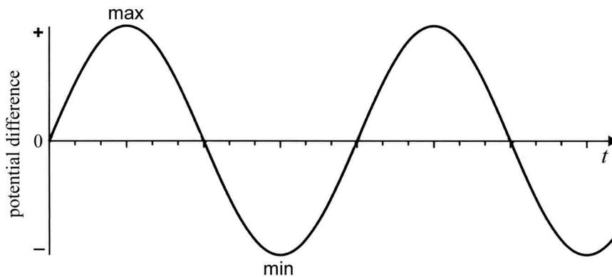
**Figure 4:** The potential difference between the terminals of a sinusoidal AC supply.
