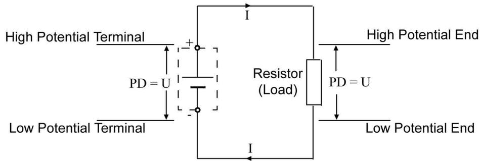
**Figure 2:** A simple AC circuit showing the potential difference (PD) across the battery terminals and the resistor.
