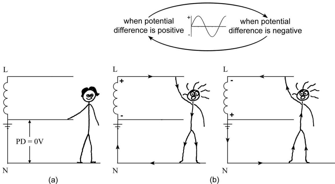
**Figure 7:** Shock hazards from an earthed neutral circuit: (a) touching the neutral wire; (b) touching the phase wire.
