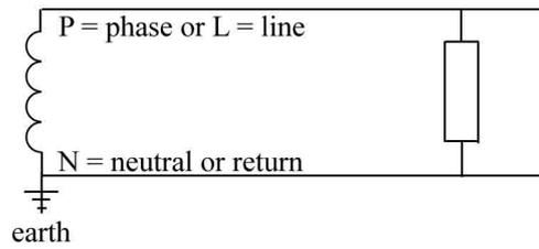
**Figure 6:** A simple AC circuit with the neutral earthed. The supply is shown as the output from the secondary coil of a transformer.
