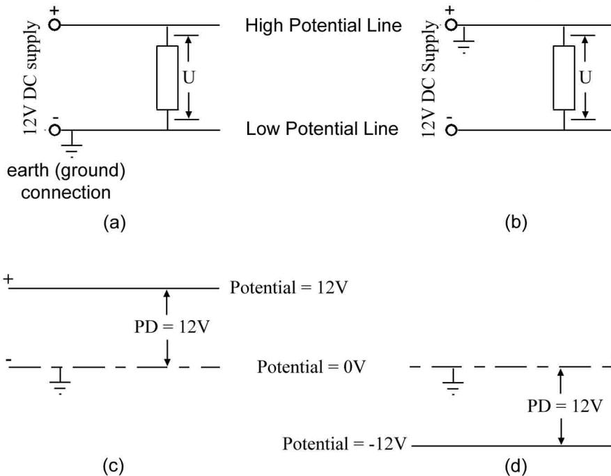
**Figure 3:** A simple DC circuit with: (a) negative line grounded; (b) positive line grounded; (c). Also the potential and potential differences with: (c) negative line grounded; (d) positive line grounded. Notice that in both instances the potential difference (PD) is 12V.
