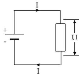
**Figure 1:** A simple DC circuit containing a battery and a resistor.
